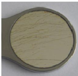
Fig. 3 Scratches/cleaning streaks
